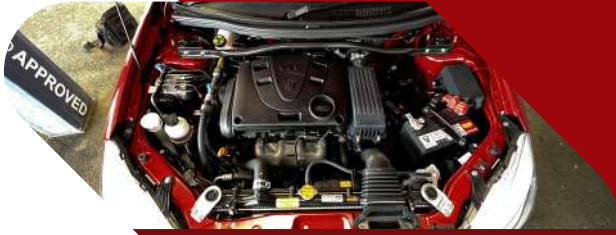
1.3L, 4 Cylinders In-Line, 16 Valve DOHC, VVT Petrol Engine
